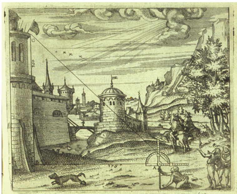
Fig. 2.5 Description of the procedure to measure heights (Zubler 1607b, 19)
