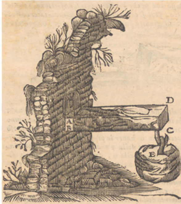
Fig. 4.1 Illustration of Galileo's cantilever model (Galilei 1655, 86)
